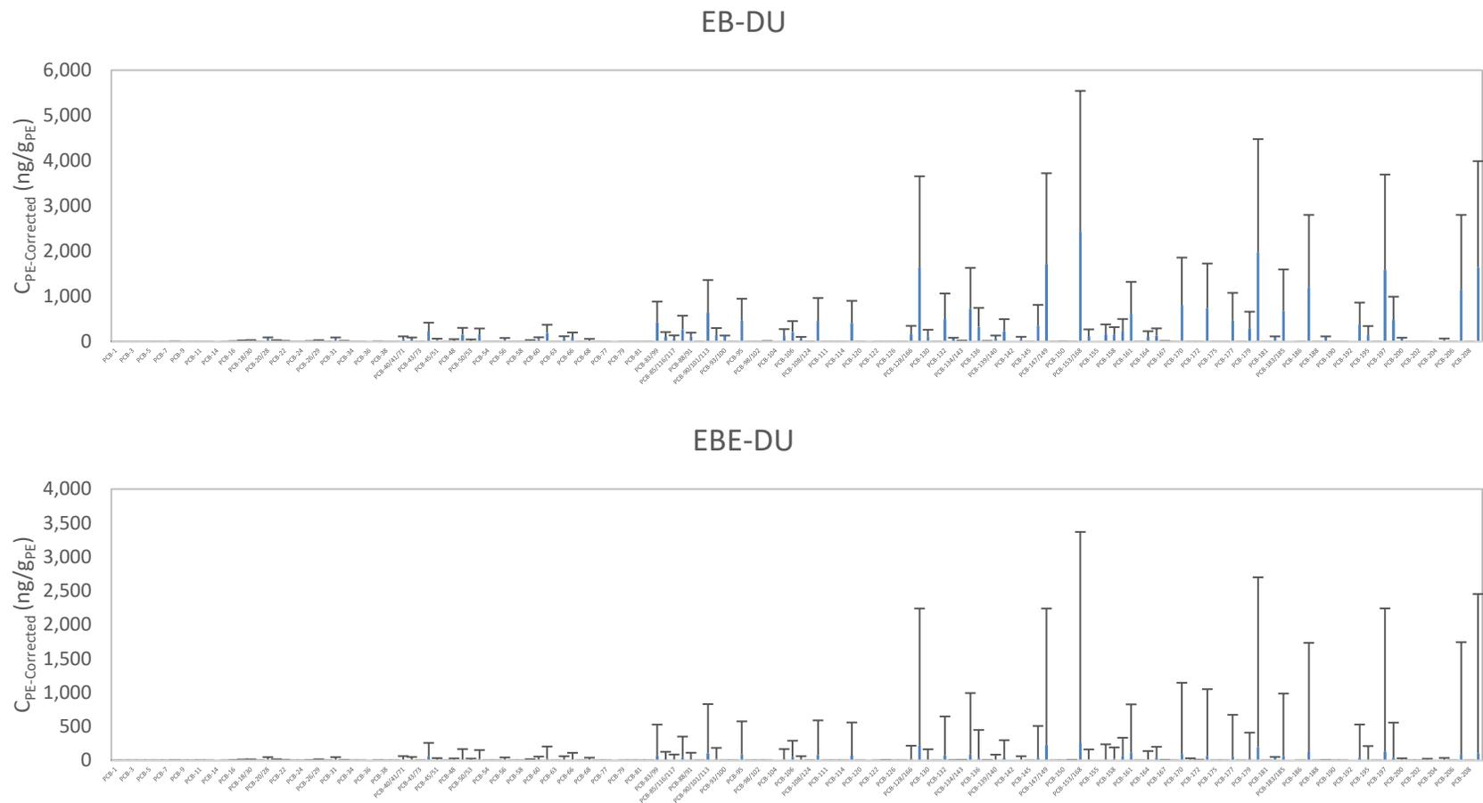
Figure 4. PRC-Corrected PE Concentrations ( $C_{PE-corrected}$ ) of PCBs Calculated from *ex-situ* experiments with PE passive samplers
