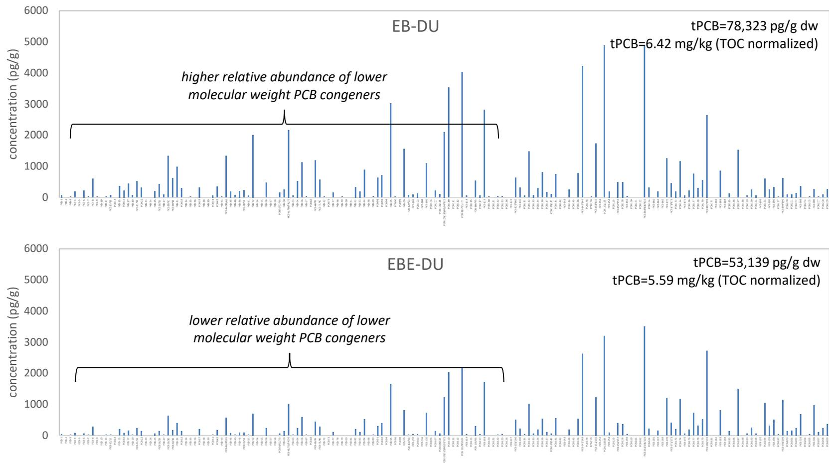
Figure 8. Concentrations of PCB congeners in EB-DU and EBE-DU surface sediment, 0-10 cm.
