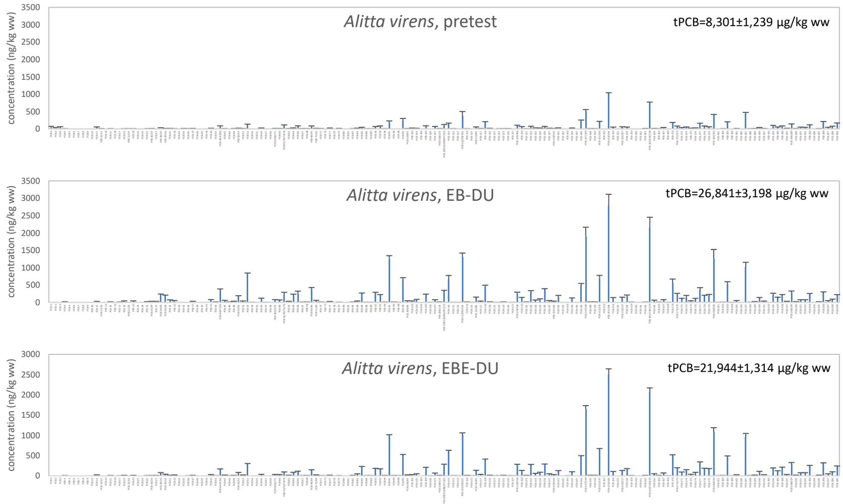
Figure 12. Concentrations of PCB congeners in *Alitta virens* following 45-day bioaccumulation tests with EB-DU and EBE-DU sediment. Figures represent average (plus standard deviation) of n=3 measurements for the pretest and n=5 samples each for the EB-DU and EBE-DU bioaccumulation tests. Data are shown on the same scale for comparison.
