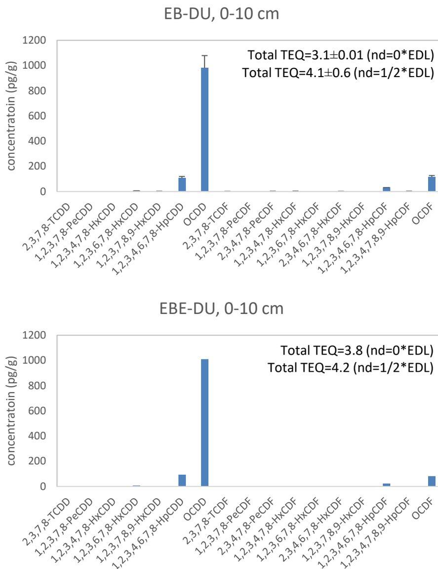
Figure 7. Concentrations of PCDDs/DFs in EB-DU and EBE-DU surface sediment, 0-10 cm. Note: the EB-DU figure (top) represents the average (plus standard deviation) of duplicate measurements, whereas the EBE-DU figure (bottom) represents a single measurement.
