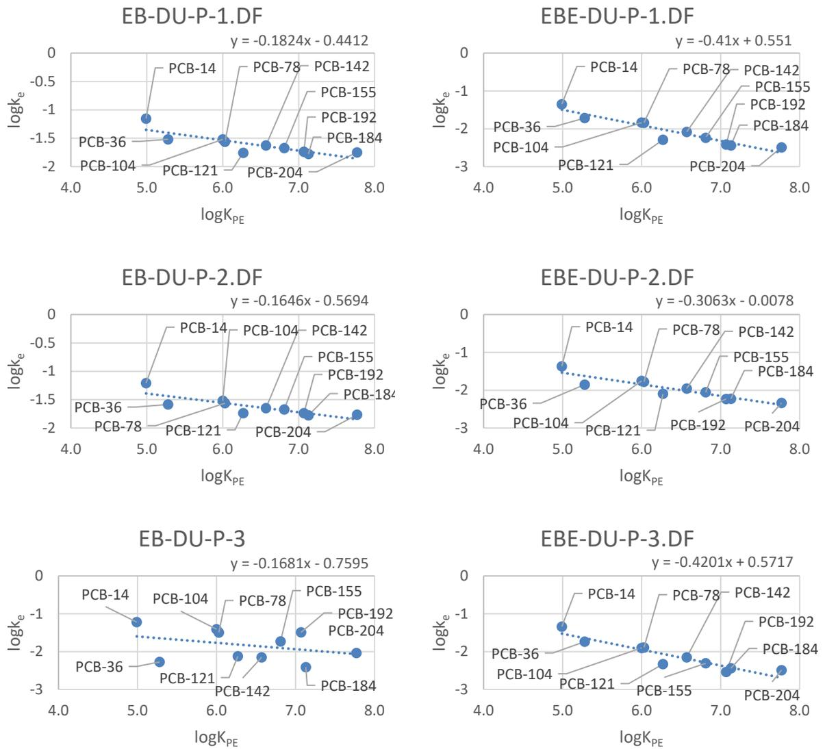
Figure 2. Relationship between  $k_e$  and  $K_{PE}$  in each of the PE ex-situ experiments for PCDD/DF measurements
