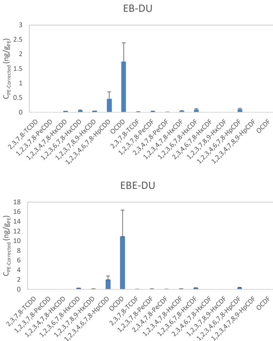
Figure 3. PRC-Corrected PE Concentrations ( $C_{PE-corrected}$ ) of PCDDs/DFs Calculated from *ex-situ* experiments with PE passive samplers
