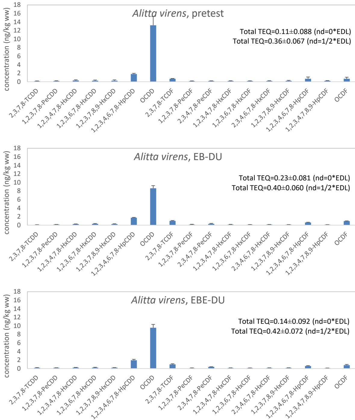
Figure 11. Concentrations of PCDDs/DFs in *Alitta virens* following 45-day bioaccumulation tests with EB-DU and EBE-DU sediment. Figures represent average (plus standard deviation) of n=3 measurements for the pretest and n=5 samples each for the EB-DU and EBE-DU bioaccumulation tests. Data are shown on the same scale for comparison.
