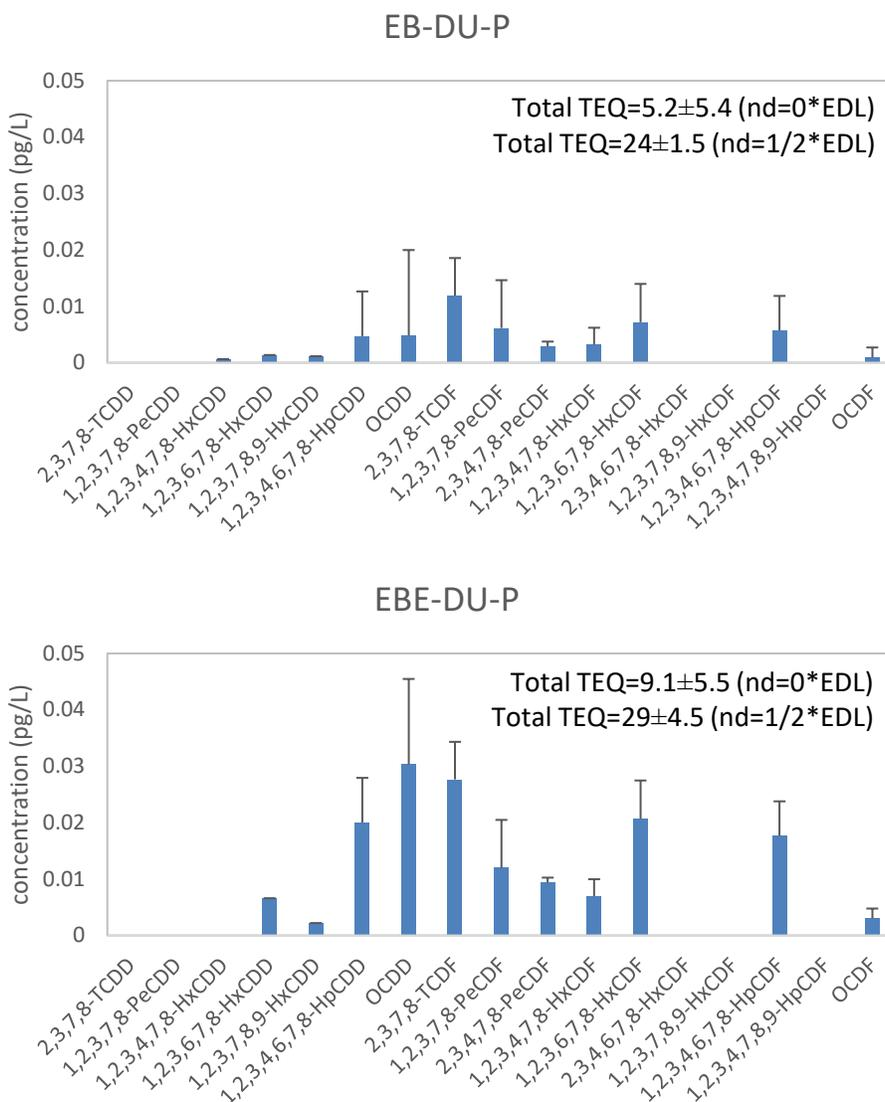
Figure 5. Porewater Concentrations of PCDDs/DFs Calculated from *ex-situ* experiments with PE passive samplers
